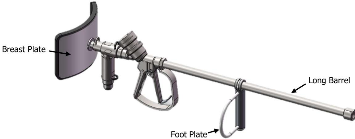
The HPE Standard Cleaning tool is the Cleaning tool that HPE recommends. This Cleaning tool can be used in both standing and sitting positions. The breast plate is used in a standing position and improves jetting control. When the Cleaning tool is used in a sitting position, the foot plate prevents the operator's foot from slipping from the foot rest and injuring the operator's legs. The long barrel assists in preventing accidental body injuries to the operator.
