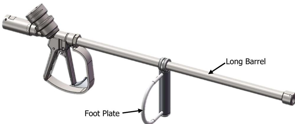
The HPE Cleaning Tool with the footplate can be used in both standing and sitting positions. Adding a breastplate will increase the amount of control the operator has. When the Cleaning tool is used in a sitting position, the footplate prevents the operator's foot from slipping from the footrest and injuring the operator's legs. The long barrel assists in preventing accidental body injuries to the operator.
